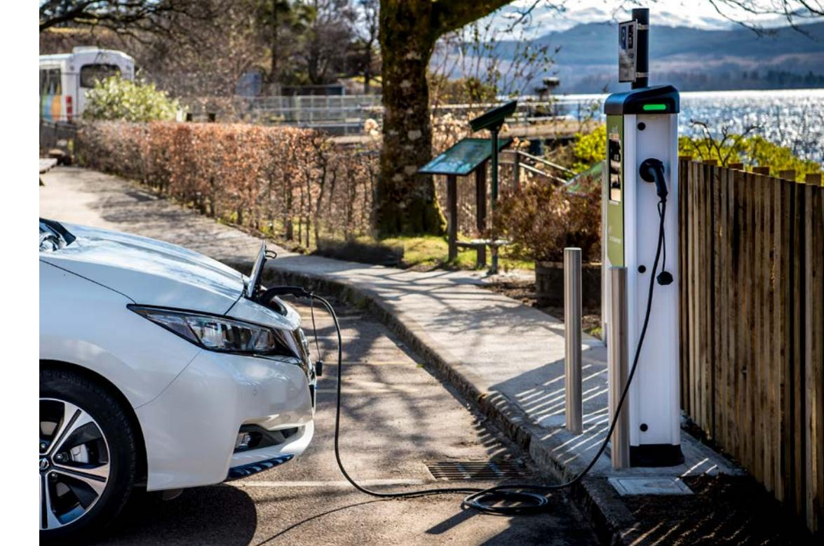
in Europe and the United States of America and is used by all European vehicles that have 'rapid' charging capability. The CCS connector incorporates a Type 2 AC connector, so only a single charging port is required on the vehicle for both DC and AC charging, enabling public, home and workplace charging.
