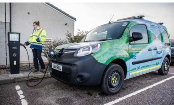
is a post, which are good on-street options but usually have higher installation costs due to the need to get the electricity to the post under the ground.
